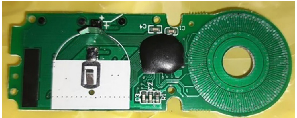
Fig. 5. The Chinese digital protractor ruler PCB
