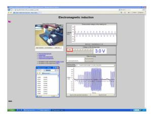
Figure 4. The web page on the client computer of the real remote experiment Electromagnetic induction with life web camera view, frequency controls, and graph of the measured data (upper plate: red - driving force, green - instantaneous deflection).
