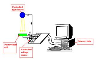
Figure 2. The schematic representation of the server of the remote experiment "Photovoltaic cell " using the system ISES <u>http://kdt-4.karlov.mff.cuni.cz/vacharakteristika\_2\_en.html</u>
