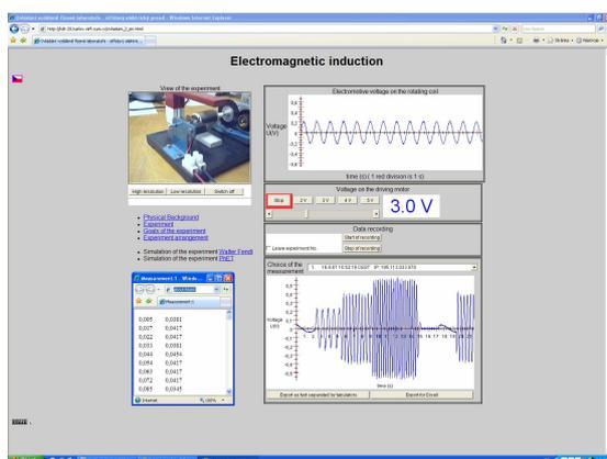
Figure 4. The web page on the client computer of the real remote experiment Electromagnetic induction with live web camera view, frequency controls, and graph of the measured data (upper plate: red - driving force, green - instantaneous deflection).
