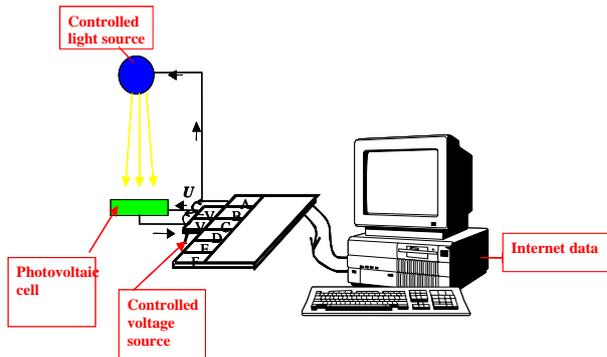
Figure 2. The schematic representation of the server of the remote experiment “Photovoltaic cell” using the system ISES [http://kdt-4.karlov.mff.cuni.cz/vacharakteristika\\_2\\_en.html](http://kdt-4.karlov.mff.cuni.cz/vacharakteristika_2_en.html)
