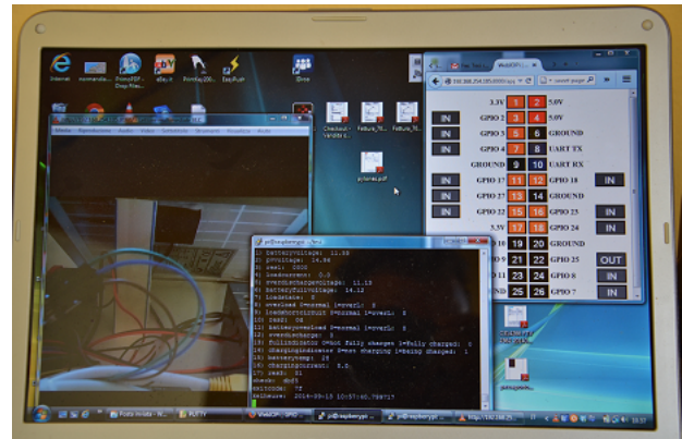
Figure 5. Photovoltaic system lab testing: video streaming (left), script controlling the Raspberry Pi and monitoring the voltages and currents (centre), microcontroller gates (right).
