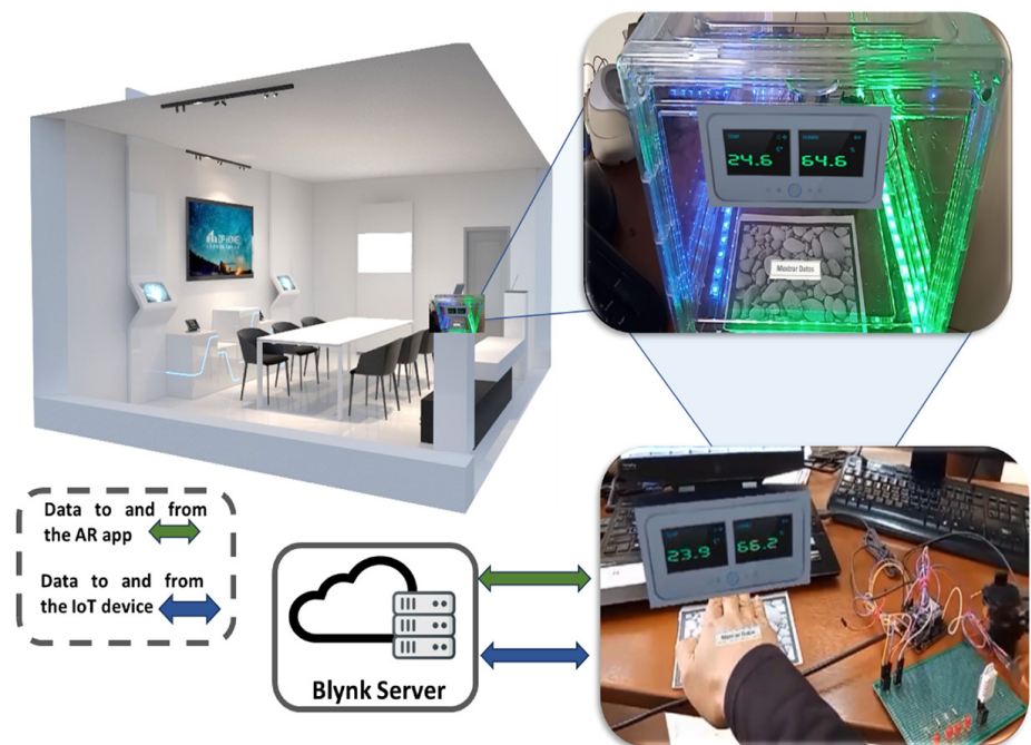
Fig. 8. AR app view showing real-time data visualization and motor control
