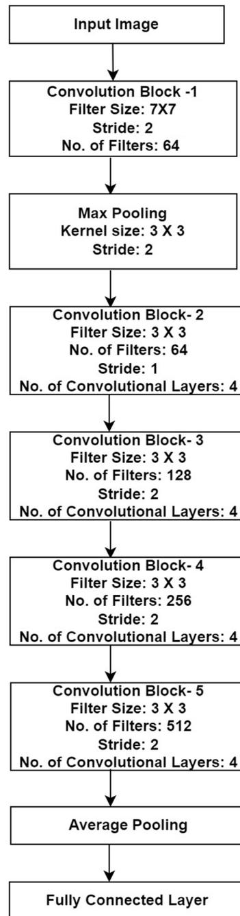
Fig. 3. Architecture of ResNet-18
