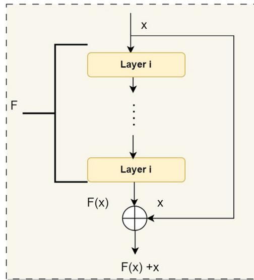
Fig. 2. Residual connection
