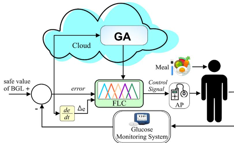
**Fig. 4.** Block diagram for the proposed fuzzy logic-based controller for type 1 diabetes patients
