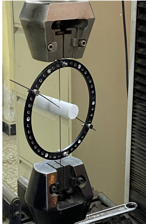
Fig. 6. Wire tensioning by computer-controlled electronic universal testing machine of max load 50KN
