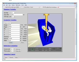
Figure 8. Portlet to simulate a synchrotron beamline X-ray diffraction instrument .
