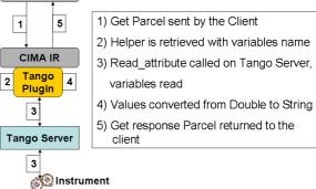
Figure 3. TANGO instrument control system as a CIMA plugin.
