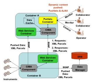
Figure 1. Remote instrument control elements. Only one person at a time can control any given instrument.
