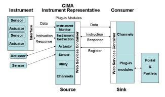
Figure 2. CIMA based components: Source components reside in Container B and the Sink components are located in Container A (see also Fig 1).
