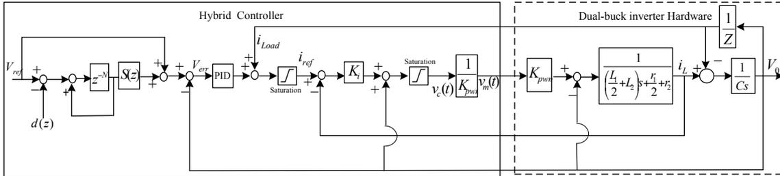
Fig.3 Block diagram of proposed hybrid control for AC voltage regulation
