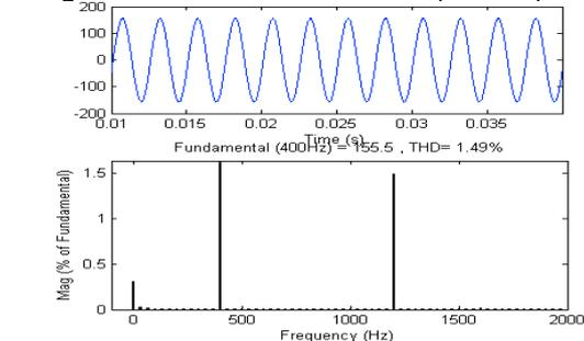
Fig.12 400Hz output spectrum at full rectifier load
