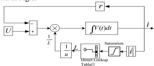
Fig.8 Inductance saturation characteristic simulation model
