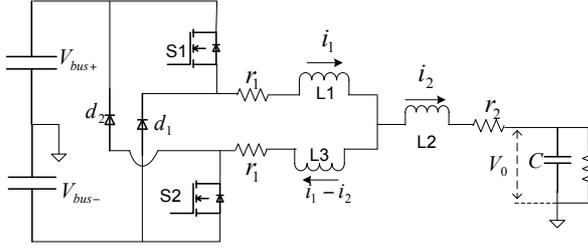
**Fig.1 Improved dual buck half bridge inverter**
