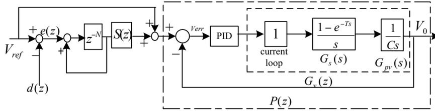
Fig.6 Simplified block diagram of the outer voltage loop
