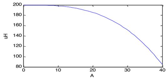
Fig.5 Nonlinear relation between the inductor current and inductance
