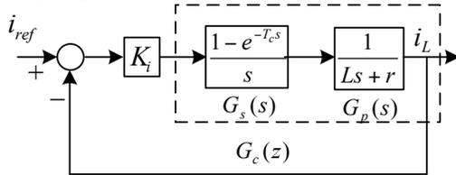
Fig.4 Simplified block diagram of the inner current loop
