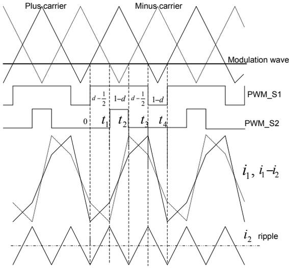
**Fig.2 Two switching duty sequence and inductor current waveforms**
