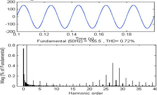
Fig.11 50Hz output spectrum at full rectifier load
