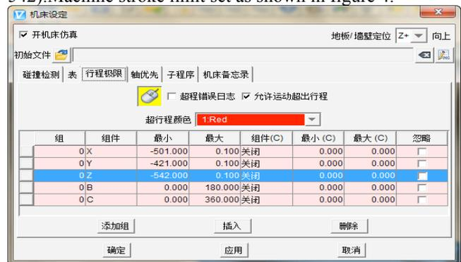
Figure 4. Machine limits set itinerary
