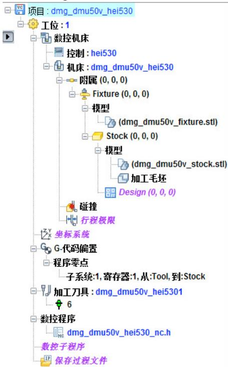
Figure 2. DMU50 component tree
