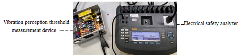
Fig. 14. Electrical safety test with the Fluke ESA 612 Electrical Safety Analyzer
