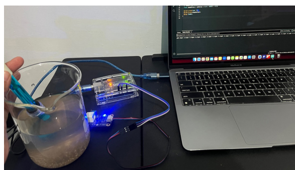
Fig. 12. Real circuit of pH sensor to Arduino and computer system
