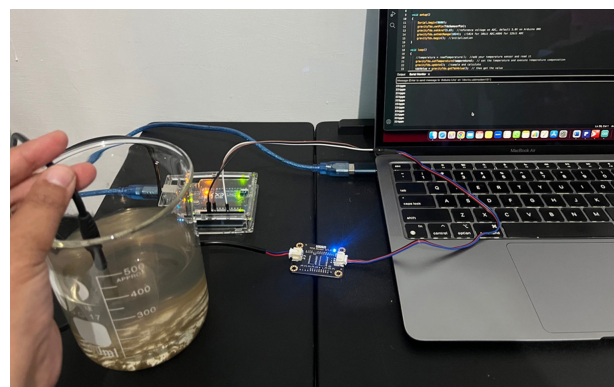
Fig. 10. Real circuit of TDS sensor to Arduino and computer system
