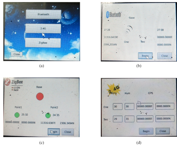
Figure 13. QT programming interface: (a) main interface, (b) Bluetooth interface, (c) Zigbee interface, and (d) 2.4 GHz interface
