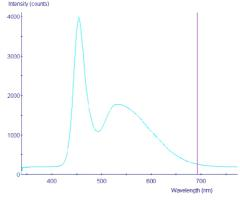
Figure 2. Spectrum of the White LED
