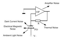
Figure 8. Noise in the Photoelectric Signal Amplifying Circuit
