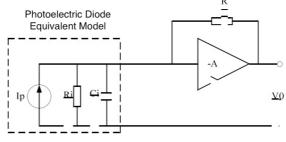
Figure 10. Transresistance Amplifier Equivalent Model
