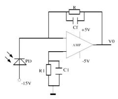
Figure 11. Adopted Transresistance Amplifier Circuit
