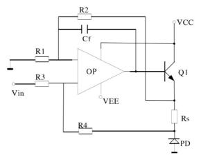
Figure 6. Constant Current Driver Circuit.
