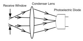
Figure 5. The Condenser Light Path of Photoelectric Diode
