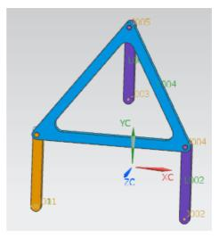
Figure 4. Simulation model of crank-group driving mechanism with clearance
