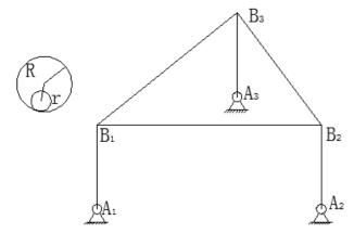
Figure 3. A diagram of the crank-group driving mechanism
