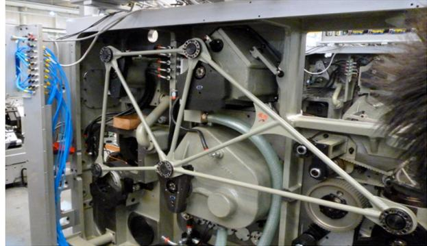
Figure 1. The application of the crank-group driving mechanism in the tobacco machinery
