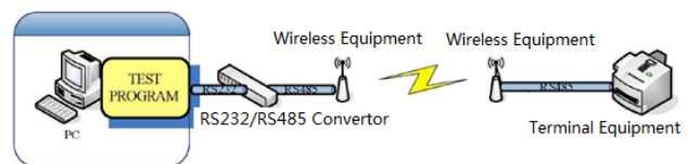
Figure 1. system basic structure
