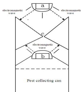
a is radar sensor, b is node of LED insect-trapping lamp
