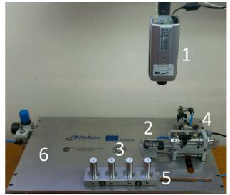
Figure 1. 1. IP web camera, 2. measurement device–digital caliper, 3. measurement object-axles, 4. cylinders for movement of measurement device, 5. axles carrier, 6. platform.
