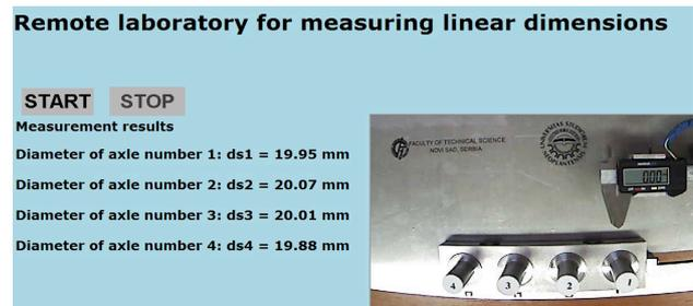
Figure 5. E-lab web client page, with camera and measuring results
