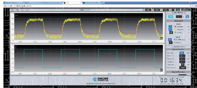
Figure 7. Real and simulated speeds of the DC Motor shaft after controller parameters calculation
