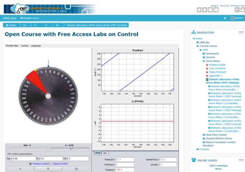
Figure 2. Demonstration of “Virtual Laboratory of the Servo Motor” (UNILabs, screenshot was made from UNILabs site [22])
