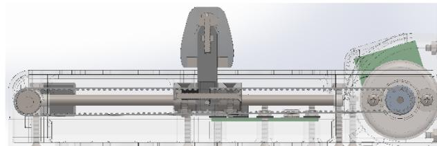
Figure 1. Side cross-section of the device, modeled in CAD software
