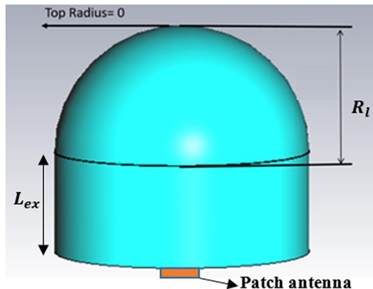
**Fig. 2.** Proposed EHS lens combined with a patch antenna
