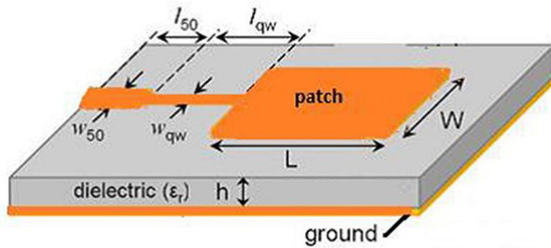
Fig. 1. Typical design of a QWT matched patch antenna
