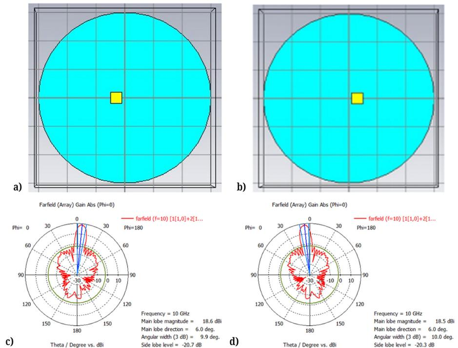
Fig. 7. At 10 GHz frequency and RT Duroid 5880 substrate, MPA array design with lens and shifting of array to a) left and b) right sides of the lens center; and observed simulated 2D radiation pattern (combined array) with c) left shift  $d_s = -\lambda_v/2$ , and d) right shift  $d_s = +\lambda_v/2$
