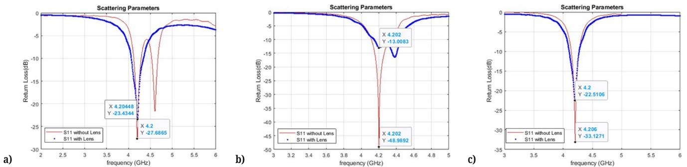
Fig. 3. The obtained return loss (S11) at frequency 4.2 GHz with and without a lens antenna using a) FR4, b) RO4350b, and c) RT Duroid 5880 substrate
