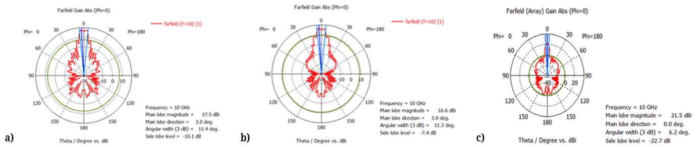
Fig. 6. The proposed 10 GHz lens antenna’s obtained 2D radiation pattern using a) FR4, b) RO4350b, and c) RT Duroid 5880 substrate
