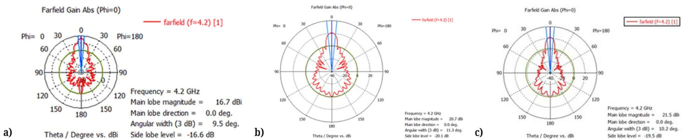
Fig. 4. The proposed 4.2 GHz lens antenna's obtained 2D radiation pattern using a) FR4, b) RO4350b, and c) RT Duroid 5880 substrates
