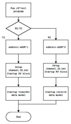
Figure 5. rf\_test1 block diagram
