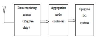
Figure 3. Receiving unit hardware structure diagram
