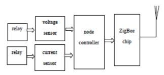
Figure 2. Acquisition of each node data's and wireless transmission structure
