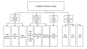
Figure 6. Schematic diagram of the computer software
