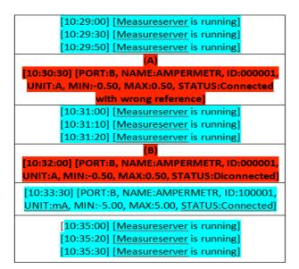
Figure 5. Remote experiments diagnostics II record, correctly running (green) and two faults (red) the setup of the remote experiment changed (range of A-meter) (A), one module A-meter disconnected (B)
