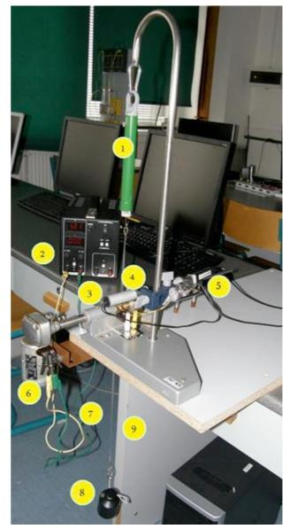
Figure 1. Joule's laboratory experiment setup (1 - the ISES dynamometer, 2 - the voltage source, 3 - a heated cylindrical metallic body, 4 - the ISES optical gate, 5 - the ISES thermometer, 6 - the driving motor (12 V; 2,2 A), 7 - leads, 8 - the loading weight, 9 - the plastic tape (photo: Z. Kratka)
