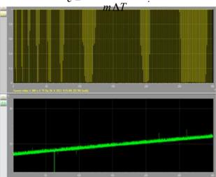
Figure 2. ISES Example of Joule's experimental data - number of revolutions (upper graph) and the temporal dependence of the temperature increase (lower graph)
