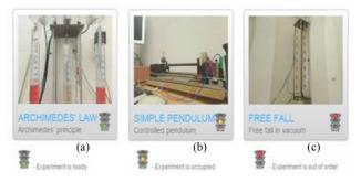
Figure 4. Remote experiments diagnostics I-the "traffic lights" signal availability of the experiment (green) (a), occupation of the experiment (orange) (b) and out of order experiment – not available (red) (c)
