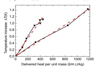
Figure 6. Specific heat evaluation: for brass ( $\mathbf{V}$ ) and aluminium ( $\mathbf{I}$ ) for various paths covered, various mass of the heated body and variousfriction forces
