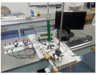
Figure 3. Arrangement of the RE "Joules' experiment"; ISES control panel (left) with the modules of the ISES thermometer, the ISES optical gate, and the ISES relay for the supply of driving motor
