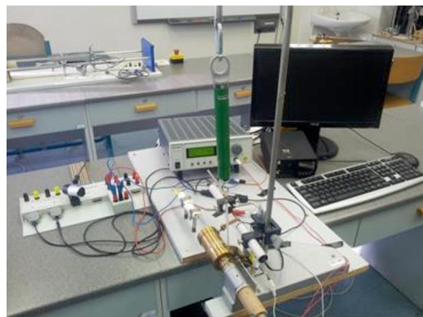
Figure 3. Arrangement of the RE „Joules' experiment“; ISES control panel (left) with the modules of the ISES thermometer, the ISES optical gate, and the ISES relay for the supply of driving motor
