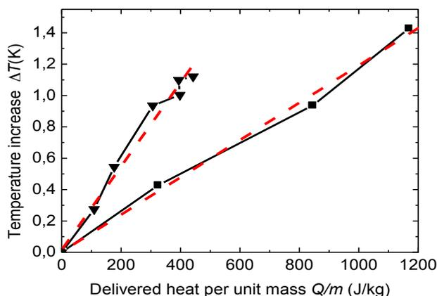
Figure 6. Specific heat evaluation: for brass (▼) and aluminium (■) for various paths covered, various mass of the heated body and various friction forces
