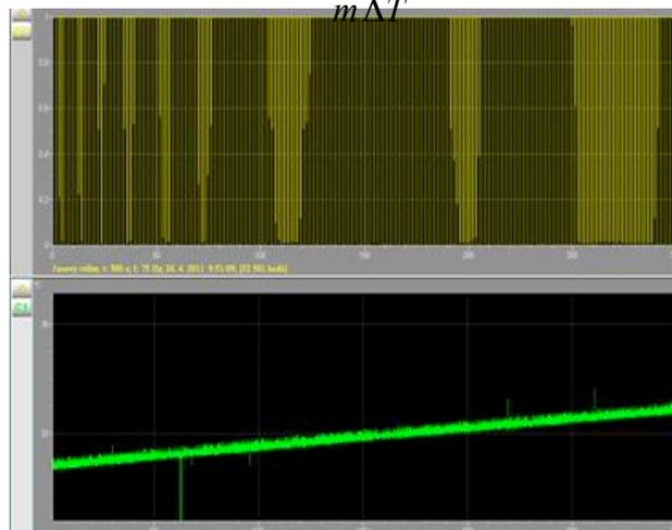
Figure 2. ISES Example of Joule's experimental data - number of revolutions (upper graph) and the temporal dependence of the temperature increase (lower graph)
