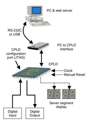
Figure 5. CPLD development board architecture
