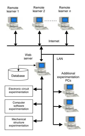
Figure 2. Remote laboratory structure (single laboratory)
