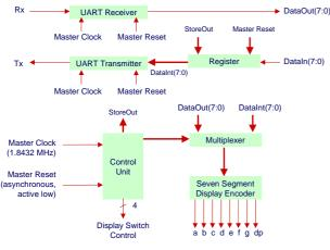
Figure 7. System block diagram
