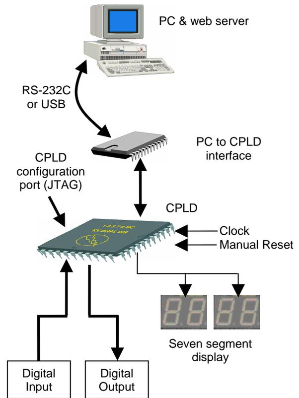
Figure 5. CPLD development board architecture
