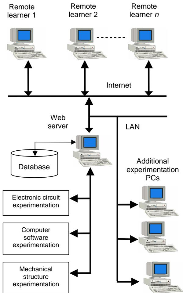
Figure 2. Remote laboratory structure (single laboratory)
