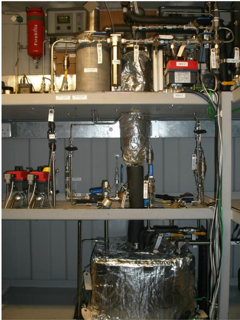
Figure 4. Photograph of the test rig, showing the solvent tank on the lower shelf, the condenser on the middle/upper shelf and most other components on the upper shelf
