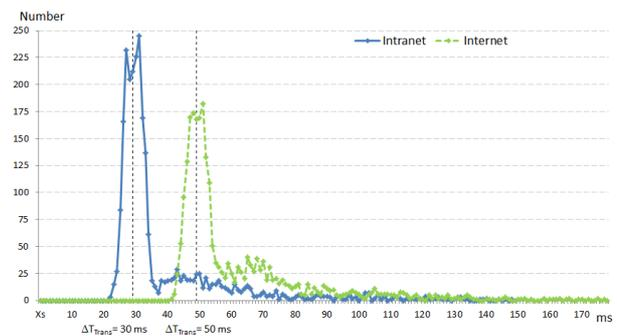
Figure 6. Time response of a bidirectional process data transmission via the Intranet (a) and Internet (b) with a PLC as I40 component
