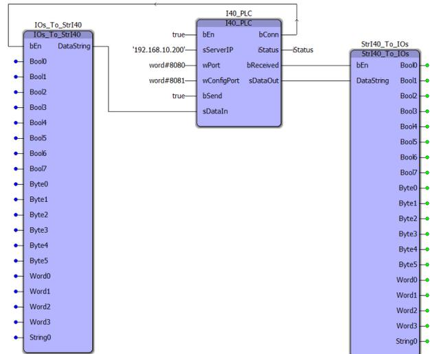
Figure 3. Prototype implementation for the device gateway as FBD program
