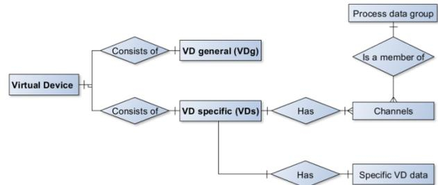
Figure 4. Data model of a virtual device
