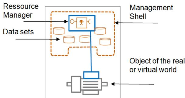
Figure 1. Component structure of an I40 component according specification RAMI 4.0 [12]
