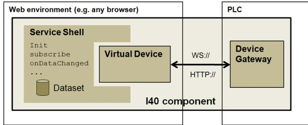
Figure 2. Model of a PLC as a I40 component
