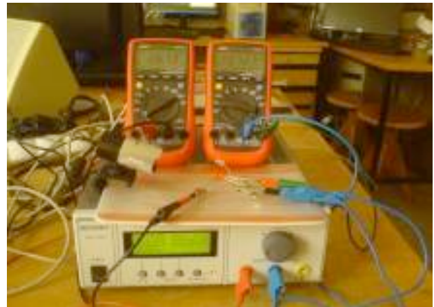
Figure 5. Power supply PSP 1405, RS232 and Multimeter UT-61E, RS232, V-A characteristics of LEDs.
