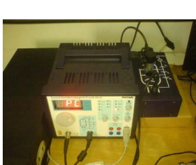
Figure 9. Phywe Franck-Hertz experiment as remote experiment Apparatus is situated at the Pedagogical faculty of Masaryk University in Brno, available on website http://147.251.192.82
