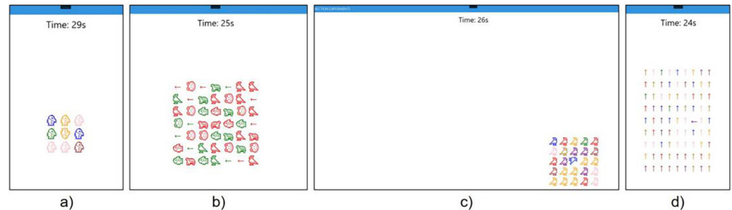
Fig. 4. User Interface of the directional experiment, with different setup examples: a) base case, 3×3 grid, all symbols, all colors; b) random group symbols, 7×7 grid, all symbols, limited colors (red and green); c) random placement of the grid on the screen, a 5×5 grid, and all symbols and all colors; d) random position of the symbol of interest, 9×9 grid, single symbol (arrow), all colors
