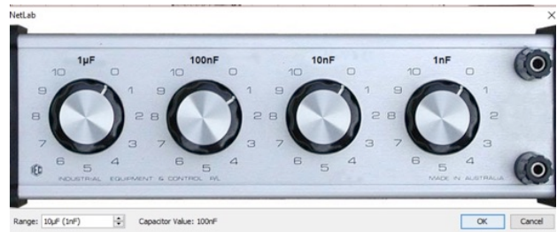
Figure 2. The 10µF range variable capacitor set at 100nF
