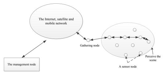
Figure 1. The architecture of wireless sensor network
