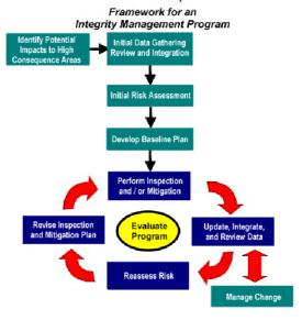
Figure 3. Pipeline integrity management framework
