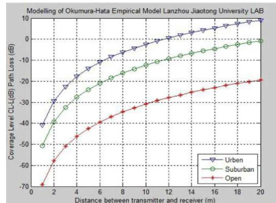
Figure 6. Restricted power of GSM and RFID at distance d (CL-L(dB)), Pathloss.
