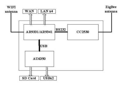
Fig. 4. The Hardware Principle of Home Gateway Host
