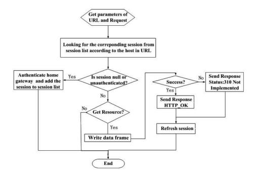
Fig. 3. The Uploading Request of Video Data Frame
