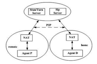
Fig. 6. The Network Topology of P2P connection
