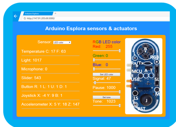
Fig. 6. Web page with Esplora sensors and actuators
