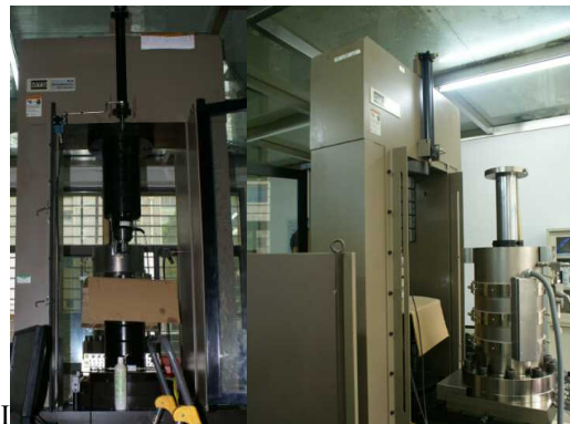
Figure 1. MTS815.04-type rock mechanics test system
