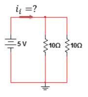
Fig. 6. Schematic of sample Ohm's Law experiment specification
