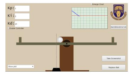
Fig. 8. Client interface for Ball and Beam Remote Lab
