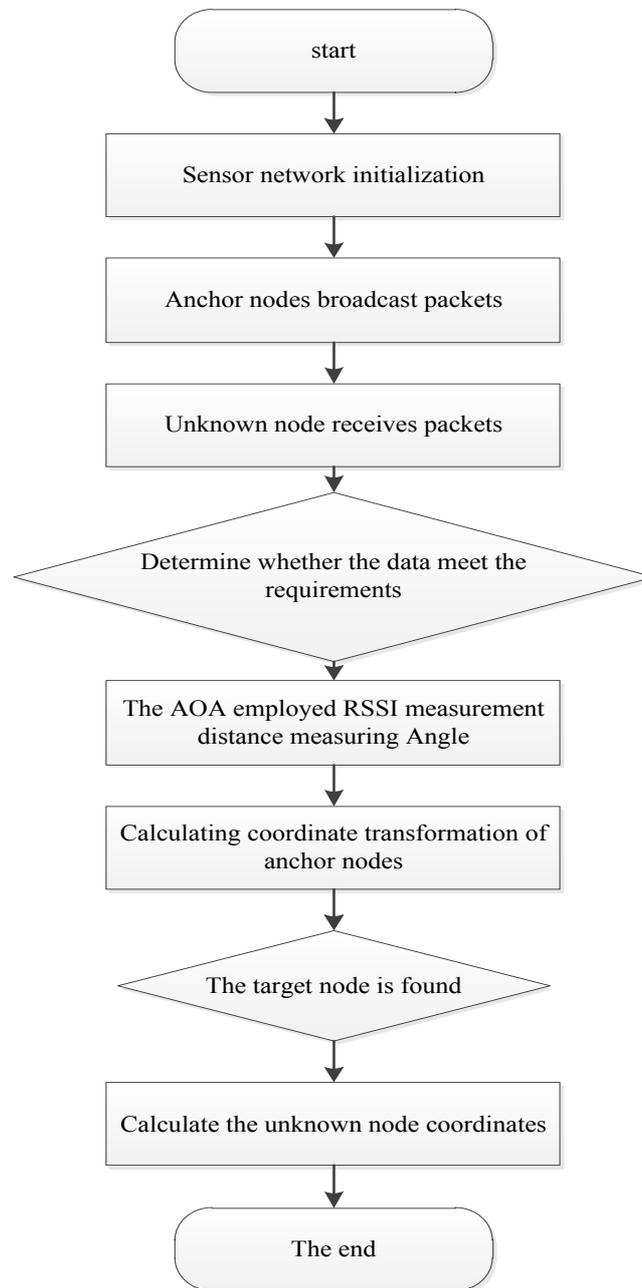
**Fig. 3.** The flowchart of the improved algorithm
