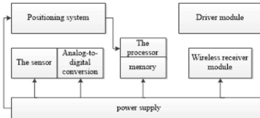
Fig. 2. The hardware structure of WSN
