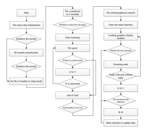
Fig. 4. The flowchart of the terminal program
