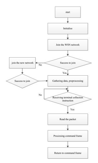
Fig. 3. The software flowchart of wireless sensor node
