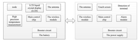
Fig. 2. The hardware design of the recorder
