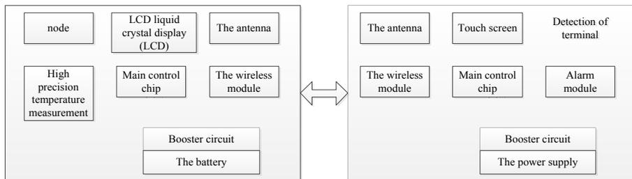
Fig. 2. The hardware design of the recorder
