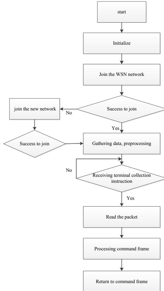
**Fig. 3.** The software flowchart of wireless sensor node
