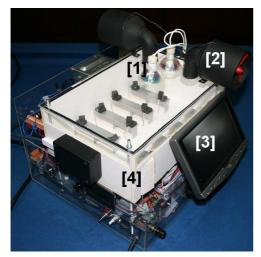
Figure 2. Final look of the scale model [1- Heating actuators, 2-Cooling actuators, 3- Touch screen display, 4- Disturbance (door)]
