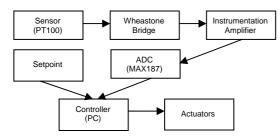
Figure 1. Block diagram of the project
