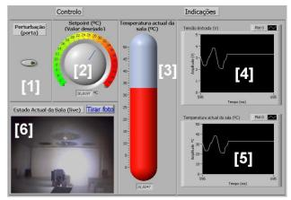
Figure 4. Application interface [1- Disturbance (door) activation button, 2- Setpoint adjustment, 3- Classroom temperature (°C), 4- Input voltage over time (V), 5- Temperature over time (°C), 6- Webcam display]
