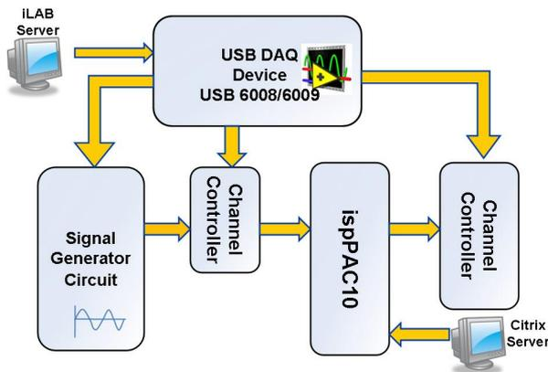
Figure 2. The Remote Lab ispPAC10 Analog Circuit.
