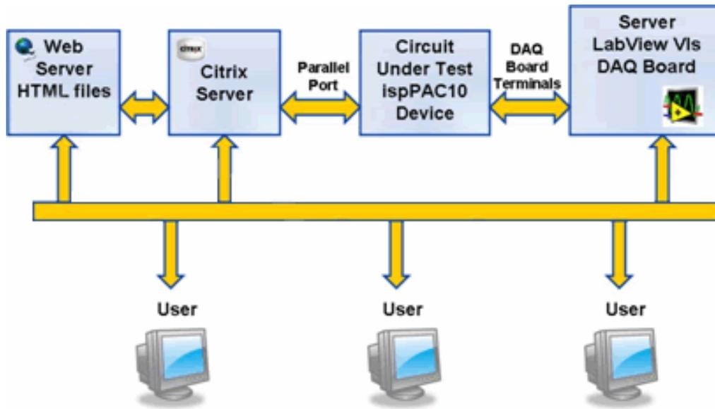
Figure 3. The Remote Electronic Laboratory System.
