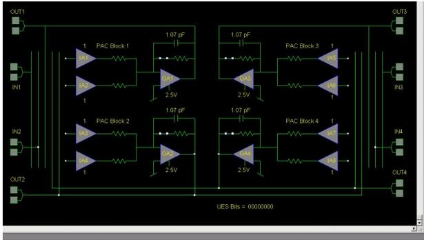
Figure 1. Basic Building Block of the ispPAC10.
