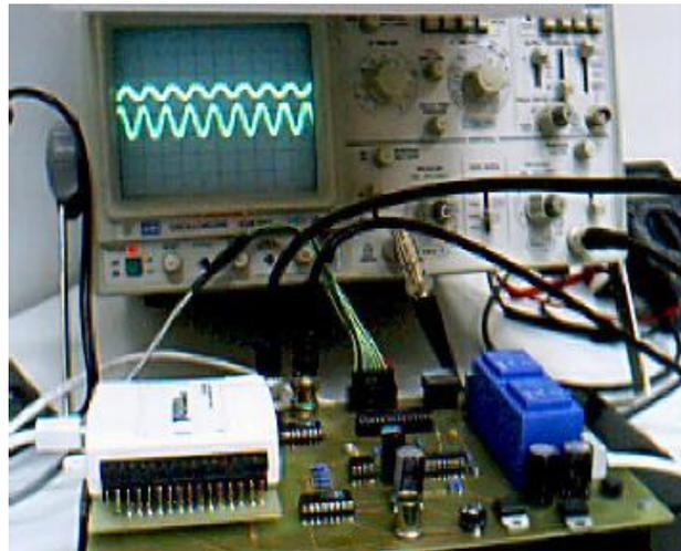
Figure 5. The iLab ispPAC10 Analog Circuit Board, showing the NI DAQ card.
