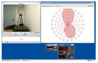
Figure 5. Running laboratory session, to the right is the software program for the tat antenna techniques and to the left is the remote controlled camera.
