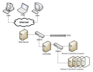
Figure 6. Expanded system with more homogenous RCC.
