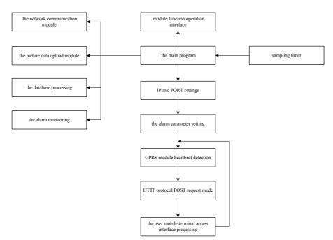
Fig. 7. Control software program structure diagram
