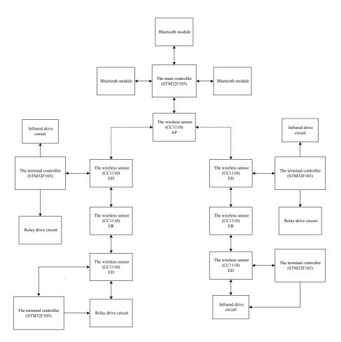
Fig. 2. Hardware system design structure
