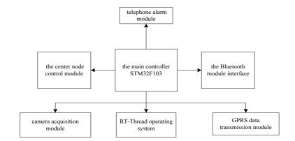
Fig. 3. The main controller system function frame diagram
