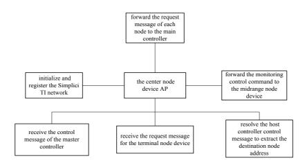
Fig. 5. The central node design block diagram
