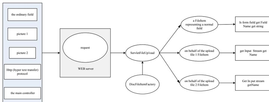
Fig. 8. Picture upload server implementation diagram
