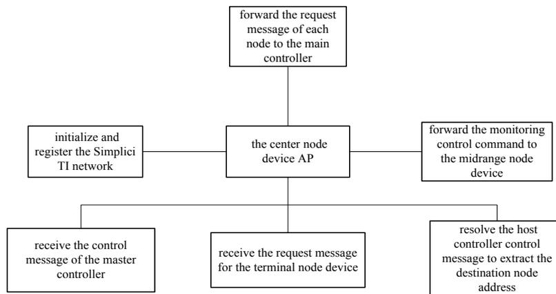
Fig. 5. The central node design block diagram
