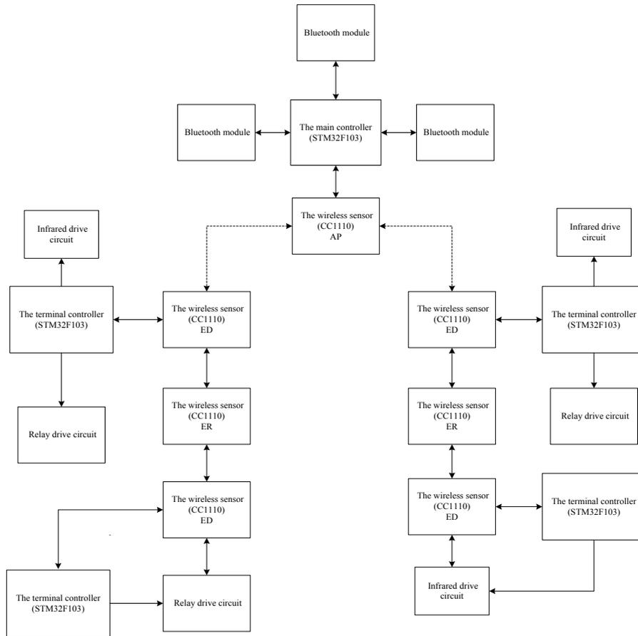
Fig. 2. Hardware system design structure
