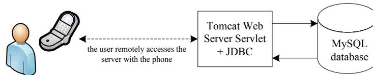
Fig. 11. The information test program of mobile phone browsing remote server image
