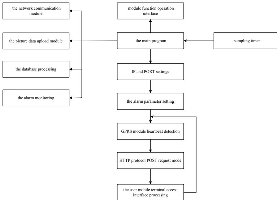
Fig. 7. Control software program structure diagram
