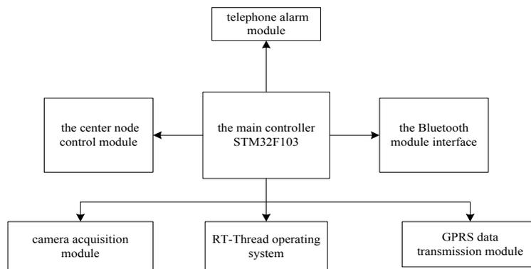
Fig. 3. The main controller system function frame diagram
