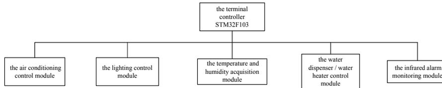
Fig. 4. The terminal controller function frame diagram
