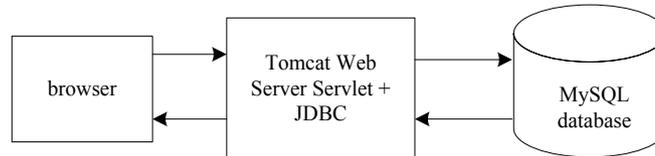
Fig. 9. Picture upload plan based on the Servlet + JDBC technology
